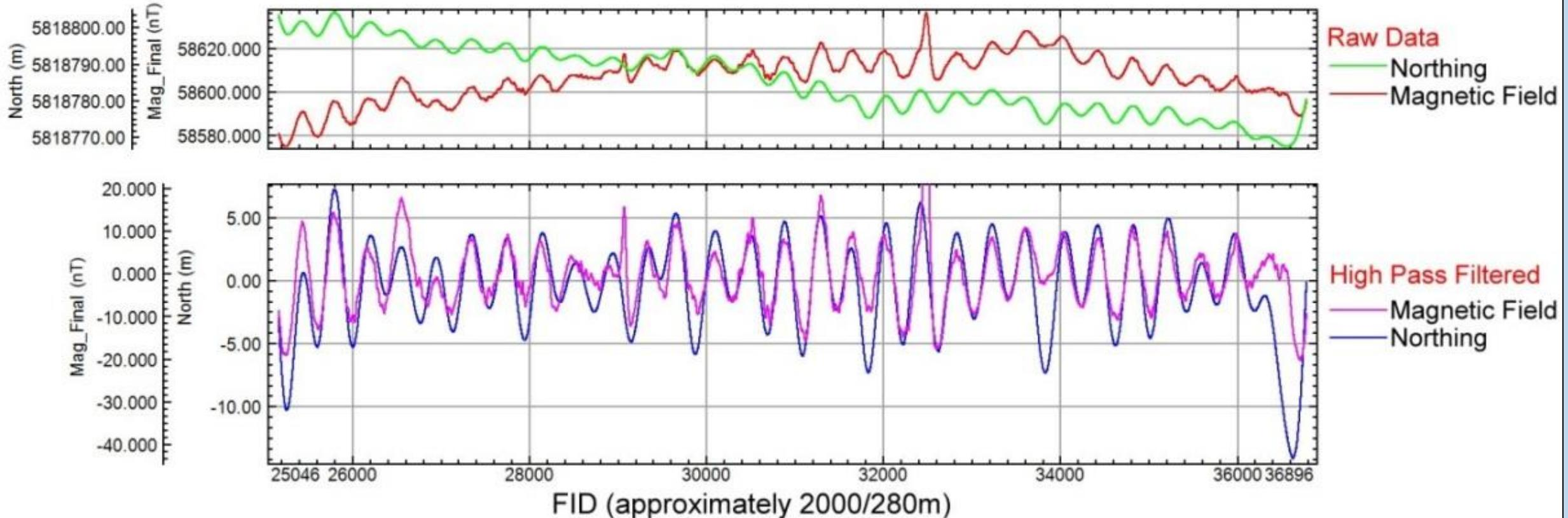
*Example of an E-W line flown with a Fluxgate system flown under very windy conditions. The top panel shows the recorded magnetic data (red) and the north position of the sensor with the respective high-pass filtered version in the bottom. [Source: Paul Mutton – Touchstone Geophysics]*
